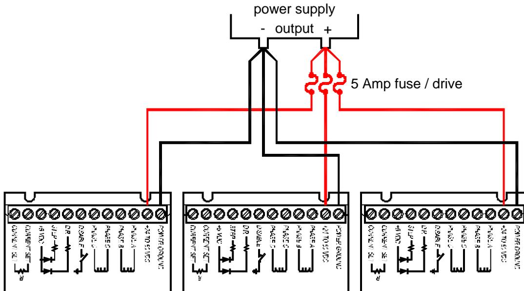
When using multiple drives from a common power supply, use individual supply and ground wires to each drive and return them to a common point back at the power supply. This is called a “star” power supply distribution; never ever use a “daisy-chain” power distribution, where the supply and ground wires for the next drive are picked up from the previous one.
