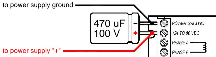
The power supply voltage must be between 24 VDC and 80 VDC. Beyond that, the choice of voltage is dependent on the application and the motor used. The power supply voltage should be between 3 to 25 times the motor's rated voltage. If it is less than 3 times, the drive may not operate smoothly and motor heating is excessive if it is more than 25 times the motor's voltage.
