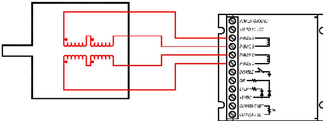
Six-wire motors are the most common. There are two connection options; full-winding and half-winding. A six wire motor is just like a four wire motor except there is a center tap on each of the two windings, for a total of six wires. For a half-winding connection, the center tap and one of the end wires are used.
