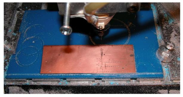
Now, although I jogged the cutter away after drilling, so I could take the previous photo, I made sure I did not reset any of the origins. I jogged the cutter up well clear of the board before moving horizontally.
