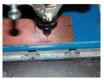
The picture below shows the situation after all the holes were drilled. You can see the crudely clamped piece of perspex, and the fact it has been used before. You can also see that it would be tricky to fit a locating pin into this material, so I didn't!
