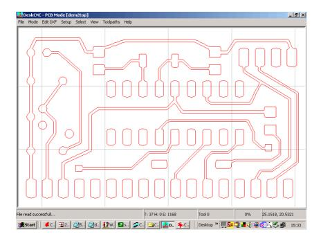
We now need to position the origin pad, at the origin of the DeskCNC workspace, so we open the 'scale, move and rotate window', and enter the required offsets, -8 and -10. No, it didn't work for me either!
