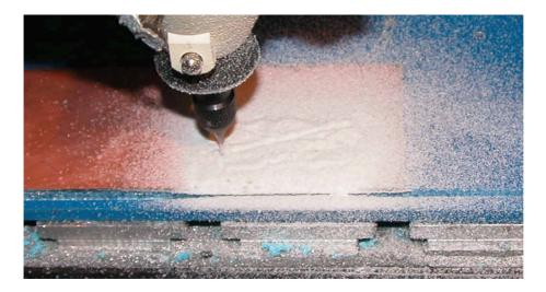
To mill the bottom side of the PCB, required its removal form the perspex backing plate, turning over, and sticking back down again.
