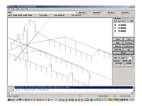
One other Deskcnc gotcha. I have a number of PCs with DeskCNC installed, not all are at the same version number. When installing a new version, sometimes I do not correctly install the milling machine setting values. If I display this .DNC file in a machine set to four axis, then I get no visible changes in the y axis screen plot direction, the holes look as if they would be drilled in a row parallel with the x axis.
