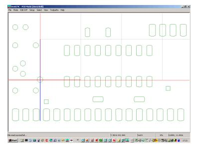
.The drill function menu is not accessible if you have loaded a Gerber file, so you need to save this file as a .dxf file and reload it. Go to 'File' menu, then 'Save Geometry DXF', then 'File', 'Open DXF', and reload it as a dxf file. The 'Drill' function can now be found under the 'Toolpaths' menu. Do a 'Select', 'Select All' (deselect the origin pad, if you will be using a locating pin to align the PCB) then choose 'Toolpaths', 'Drill'.
