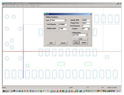
Complete the boxes, set the drill depth to be about half a millimetre or so more than the PCB thickness, and hit the 'Drill' button. Then select 'File', 'Save Tool paths CNC, and save the .DNC file.
