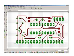
Using the CAM processor within eagle is relatively straightforward. Select the output device as GERBER\_RS274X, and enter the file name to be saved, in this instance use 'c:/demo2top'. Then select the required layers in the right hand column, so we need top, pads and vias. Check that no other layers are selected, so use menu 'layer' then 'show selected' will confirm this. Ensure 'pos Coord' and 'optimize' boxes are checked. Finally hit 'Process Job' to produce the Gerber file.
