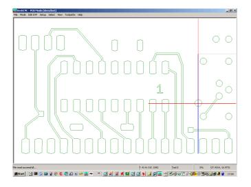
Now, we need to generate a milling .dnc file for the top layer, and also one for the bottom layer. We have previously seen how to do that in DeskCNC, so repeat the method for the top layer only, and save the file.
