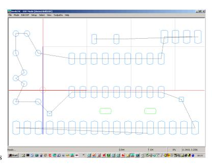
Position the cursor over the centre of the left hand diode pad, and make a note of the xy co-ordinate values. You could zoom in if you want more precision, but I make it to be X14.33, Y-4.88. Get the co-ordinates of the right hand pad, X24.42, Y-4.88.
