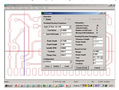
pre select the regions you work with. As this was initially loaded as a Gerber file, everything is selected. However, we do not need to mill out the origin locating pad, so deselect it, then open up the 'Toolpaths', 'Route' menu item.. As we are using a 0.8 mm slot drill, the offset will be 0.4mm. Adjusting the offset value can give thicker or thinner PCB tracks and pads, of course.
